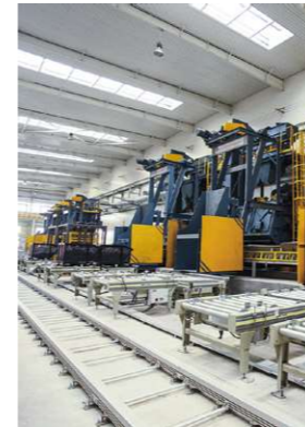
▲ Automatic Shot Blasting Process
